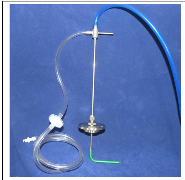
Example of a pitot tube
