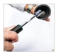
Using a 13mm soocket, unscrew the bronze dust filter and remove it from its position inside the windscreen.
