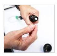
Once the windscreen has been removed, remove and discard the cellulose filter from the filter holder at the end of the wand.
