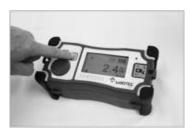
An "X" will appear over the pump icon in the upper left corner to indicate that the pump is off.
