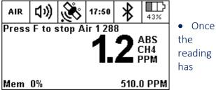
stabilized on the display, press the Function, (F) button again to stop the pump and complete Air Test 1.
