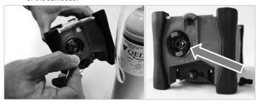
NOTE: If the tube is not fully inserted into the sample inlet of the SEM5000, the concentration readings during field calibration may appear to be erratic and difficult to stabilize.
