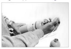
NOTE: The regulator flow must be a minimum of 0.6L/min to avoid restricting the pump. The SEM5000 package is provided with one demand-flow regulator with a C10 fitting. It is recommended that two regulators be used, (one per bottle), for ease of calibration.
