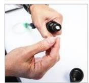
Replace the cellulose dust filter in the end of the filter holder.
