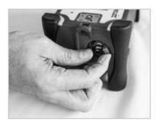
Remove filter holder by turning counter-clockwise
