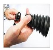
Unscrew and remove the windscreen from the end of the sample probe.
