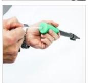
Feed replacement tubing into the handle end and push it all the way through the probe.
