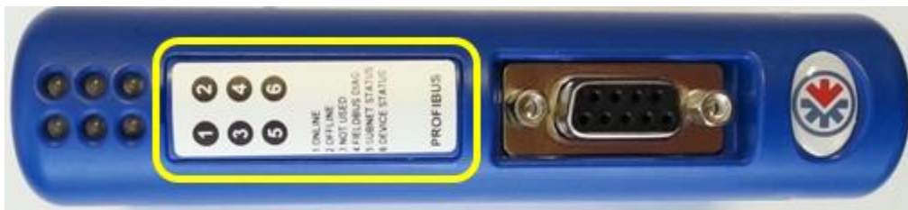
Figure 12 - Profibus module switch location
