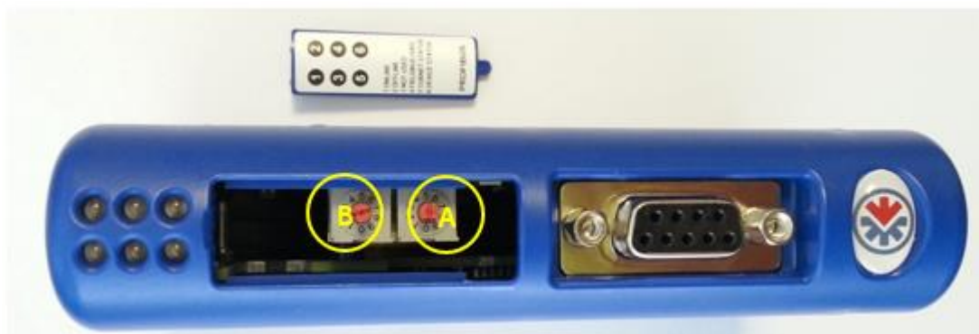
Figure 13 - Profibus module switch identification
