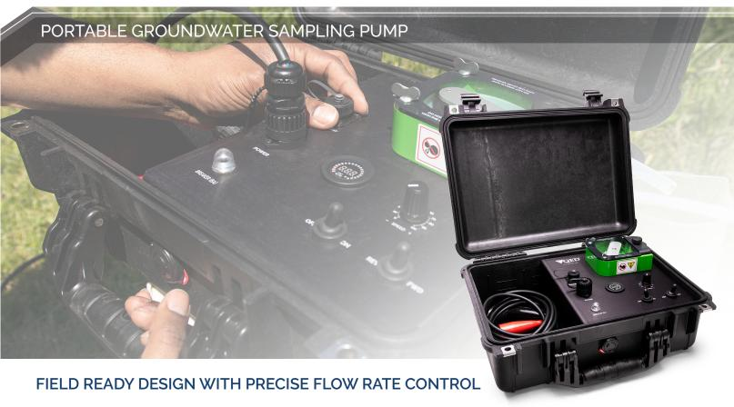
Peristaltic pumps are widely used for sampling shallow groundwater for low-flow purging and sampling. They're uniquely well suited to sampling for PFAS since the water sample only contacts the tubing in the well and around the pump head, making a PFAS-free dedicated sampling system simple and economical.
